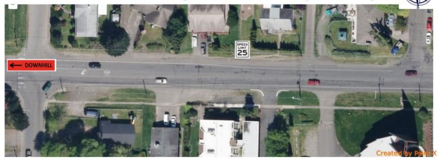
East bound lane climbs 200' elevation hill, cresting at Schley. Car lanes remain at 12'. Existing bike lane varies from 2' to 11', crumbling away at the edge in several narrow locations. They are effectively made narrower by a recent overlay which extends into the bike lane, leaving a tall lip between new and old pavement. The bike lane is not ideal, but safer than riding up hill in the car lane.
