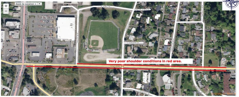
These of Sheridan have very old, crumbed and patched shoulders with a partial overlay, making riding conditions difficult and unsafe. WSCC recommends that the shoulders be repaved and any resulting lip feathered.
